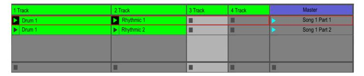
Tracks 1 and 2 are playing. The start will be done with the switch <u>7A.4. Full Start Stop Button</u>. We select the next scene and then press the Start/Stop button to chain the clips contained in the "Song 1 Part2" scene. When the "Song 1 Part2" scene is launched, the "Song 1 Part1" scene will automatically stop. This organization would allow, for example, to have a different drum set for this part.
