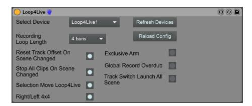
You will be able to control most parameters contained in config.ini file without restarting Ableton. Select the Loop4Live device you want to edit and change parameter as you wish.
