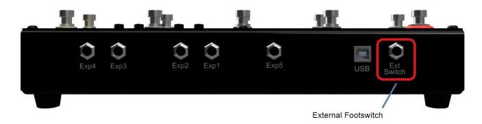
External footswitches can have 2 types of switches: either temporary or latching (guitar amplifier footswitches are most often latching). Depending on the type of switch, the EXT\_BUTTON1\_MOMENTARY and EXT\_BUTTON2\_MOMENTARY parameters in the config.ini file must be configured. These parameters set to 0 will correspond to latching switches, and conversely setting them to 1 will correspond to temporary switches (see section 6D. Loop4Live configuration in Ableton Live).
