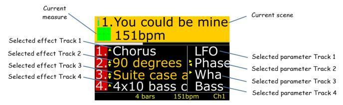
The proposed effects are those present on the 4 tracks currently selected by the pedalboard. When switching modes with Loop4Live, the first effects displayed will be the sends. Pressing the up/down buttons on the footswitch will scroll through the track effects. Pressing the Left/Right buttons will scroll through the parameters. Enabled effects are displayed in orange, disabled effects are displayed in white. The effects can be activated/deactivated with the A-B-C-D buttons:
