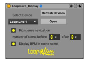
The "Refresh Devices" button refreshes the list of pedalboards in the "Select Device" drop-down list.
