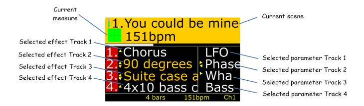
The arrows next to the effect names indicate whether it is possible to go down or up and the arrows next to the parameter names indicate whether other parameters of the same effect can be selected with the left/right buttons.
